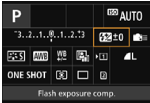
The Quick Control screen is displayed by pressing the Q button in shooting modes. Here the icon for Flash exposure compensation is highlighted and its name is displayed below. The function settings screen is identical but you cannot select or change settings.
