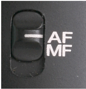
The lens focus switch can be set to AF for autofocus or MF for manual.
