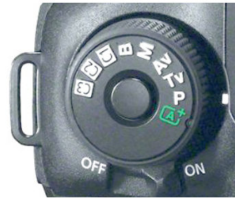
The Mode Dial can be set so you can manually select the shutter speed (Tv) or aperture (Av). To change shooting modes you hold down the Lock-release button in the center of the Mode Dial and turn the dial to align a shooting mode with the white index mark. Here it is set to the P (Program) shooting mode.
